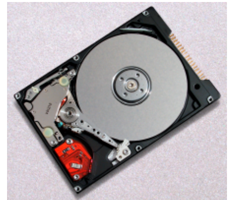
Hitachi Travelstar 40GNX: 9.5mm, 5,400rpm, 40GB ATA-5 hard disk drive 1
