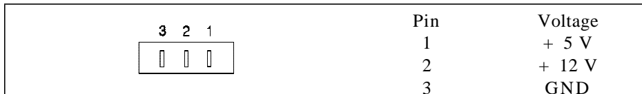
Figure 24. Alternate Power Connector Pin Assignments
