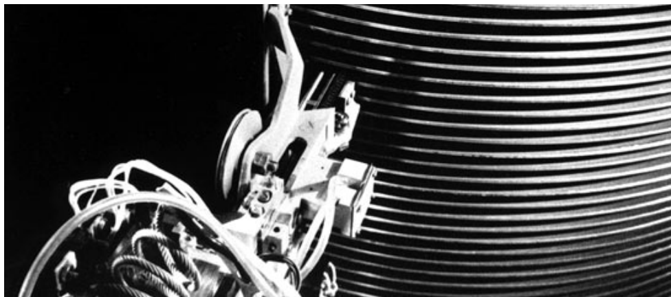
1956, RAMAC—The world's first hard disk drive stored 5MB of data on 50 24-inch disks
