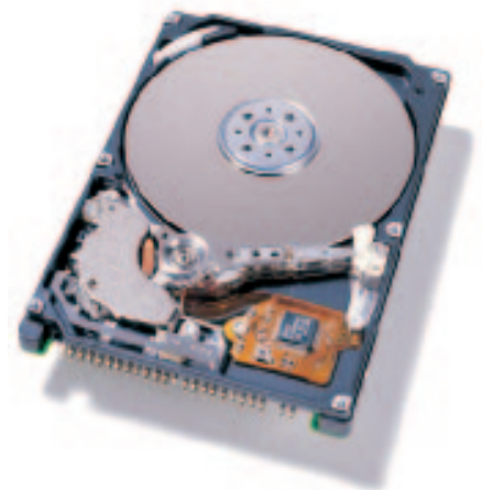
Travelstar 3GN 2.5-inch 3.2 GB ultra-low-profile disk drive
