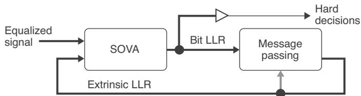
Both the SOVA and MP blocks pass information between bits. The SOVA block exchanges information between bits that are related to each other by proximity (ISI). The MP block exchanges information between bits that are related to each other by the parity check equations of the LDPC code.
