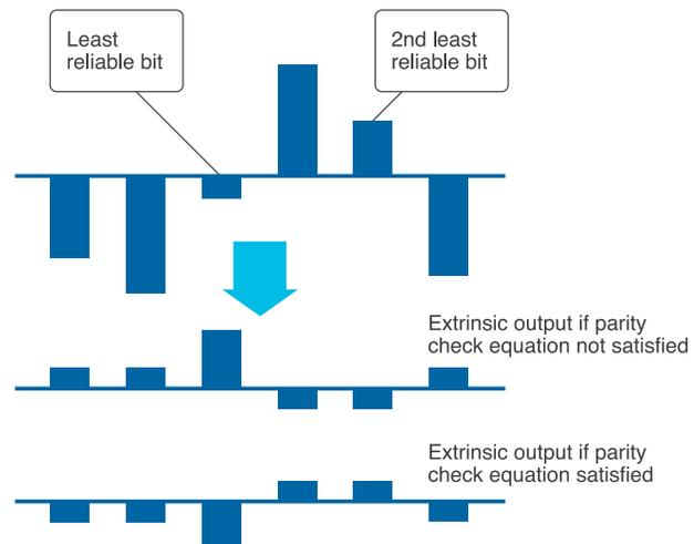
It should be noted that a parity-check equation relates a set of scattered bits by parity. The bit-to-check step can be viewed as an information-gathering function. One piece of information gathered is whether or not the parity-check equation is satisfied, and the sign of each LLR bit is used for this purpose. The bit-to-check stage also identifies the least- and second-least reliable bit locations along with their LLR magnitudes.
