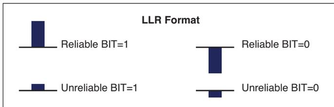
LLR values can be graphically represented by bars. Bars above the zero reference line are considered BIT=1. Bars below the zero reference line are considered BIT=0. This is illustrated in the graph to the left.
